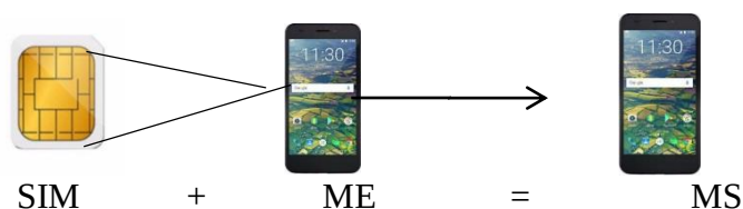
Figure 1.2: Component of mobile transceiver (activated handset) (Oluwafemi, et al. 2020).
