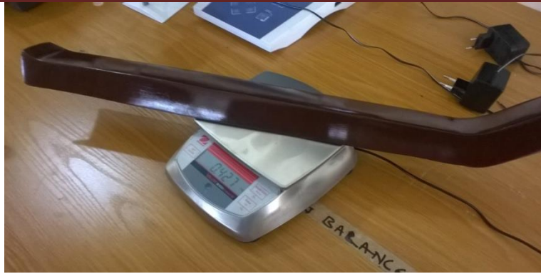
Figure 14: Finished Chassis panel weighs 421grams
